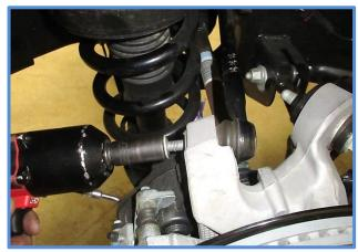
4. Remove the bolt from the other upper link using a 24mm socket (nut is welded).
