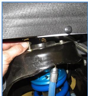
7. Place a jack under the lower control arm and raise the arm up until the shock mount in the lower control arm is in line with the shock. Install the factory bolt and tighten to factory specs. Now tighten the upper mounting bolts to 35 ft. lbs.
