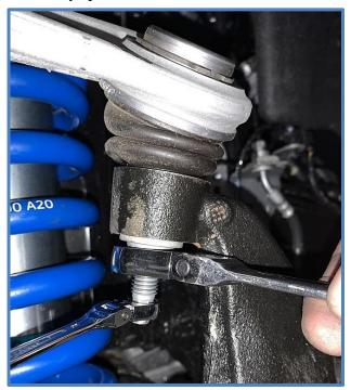
13. Now you can torque the upper and lower mounting bolts. Torque the upper bolts to 35 ft/lbs. using a 9/16 socket. Torque lower bolts to 90 ft/lbs. with an 18mm socket on the nut & 19mm wrench on the bolt head.
