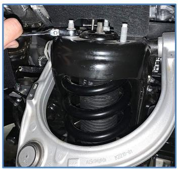
4. Separate the upper control arm from the knuckle. Using an 18mm wrench or socket remove the nut for the control arm ball joint, then disconnect upper arm from knuckle.
