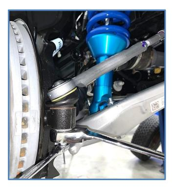
12. Reconnect the upper control arm and tighten to factory specs.
