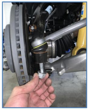
6. Disconnect the sway bar links on both sides of the vehicle. Remove the nut using a 21mm wrench, you may need to hold the stud with a hex key to keep the stud from spinning.
