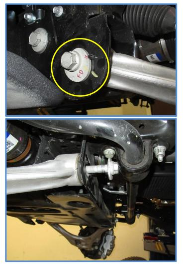
Place the lower control arm back into the lower mount and install the cam bolts to the same position prior to removal. The vehicle will need to be aligned properly after the install but keeping the factory settings will get you to the alignment shop. Tighten lower control arm bolts to factory specs after the vehicle is sitting back on the ground. Removing right shock should not require removing lower control arm bolts. Remove right shock and move to next step...
