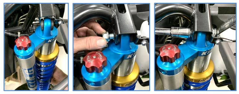
3. Place the rod end in the lower mount, install the factory hardware and tighten to factory specs.
