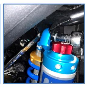
3. Place the rod end in the lower mount with the shaft guard facing forward, install the factory hardware and tighten to factory specs.
