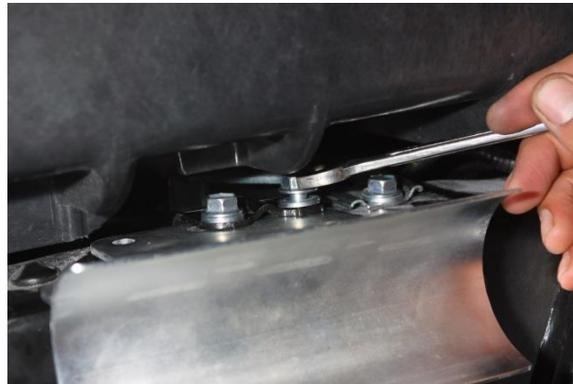
(2) On the driver's side of the truck (left), remove the bolts holding the brake line bracket to the frame as shown. Insert the reservoir bracket between the brake bracket and the frame as shown. Replace the bolts and tighten. On the opposite side (right) mount the bracket with the provided hardware using the existing holes in the frame.
