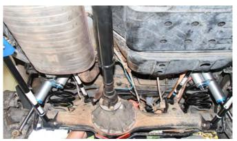
Re-install the swaybar end links and take some time to make sure the shocks and reservoirs will not contact any of the suspension links, the frame or the coil springs.
