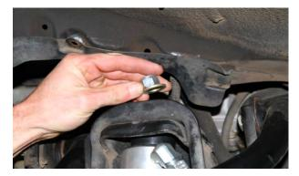
Thread nut and flat washer onto protruding pin
