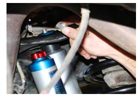
Place rubber bushing and blue annodized washer on shock pin protruding from upper shock mount.
