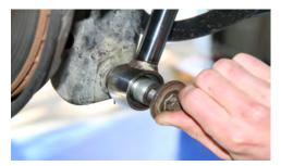
Replace factory bolt and tighten.
