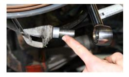
Slide bushing spacer onto lower shock mount as shown.
