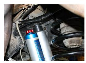
Place thick rubber bushing onto mounting pin and feed shock into upper shock mount on frame with reservoirs facing the center of truck.
