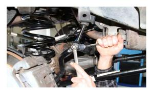
Remove swaybar link bolt on both sides of truck and drop swaybar out of way to fit shock into mounts.
