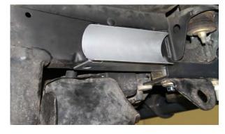
Reservoir mount attaches to the frame using existing bolts that secure skidplate and tow hook. Drop skidplate and tow hook braket, insert mount against frame and replace bolts but do not tighten. Truck shown has aftermarket bumper that requires drop down spacers that stock vehicle does not have.
