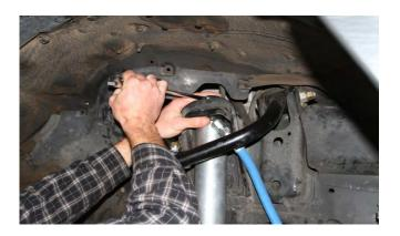
Tighten nut until rubber bushing starts to squish. Approximately 1/8" of threads on pin will be exposed. \* DO NOT OVERTIGHTEN.
