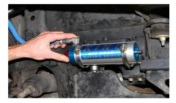
The reservoir mounts with hose fitting pointing up. Make sure hose does not interfere with moving suspension parts. Once reservoir clamps are tight, tighten remaining bolts.
