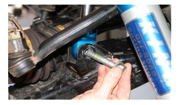
Insert rod end into lower mount and install bolt
