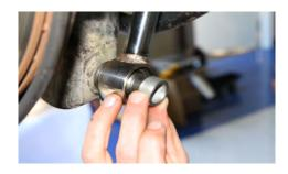
Slide rod end of shock onto mount and place bushing spacer on end of mount as shown.
