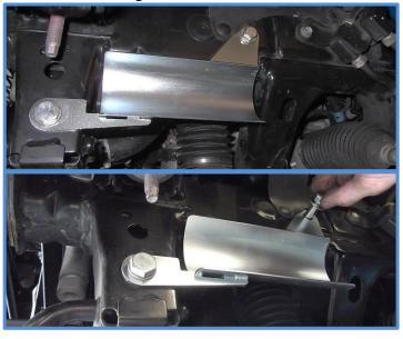
10. Install reservoir in the reservoir bracket with provided hose clamps as shown below.
