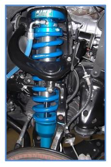
9. Install reservoir brackets using the provided hardware. Thread the 12mm bolt into the cross member, then insert the 7/16 x 3 <sup>3</sup>/<sub>4</sub>" bolt through the frame. Install washer, nut and tighten.
