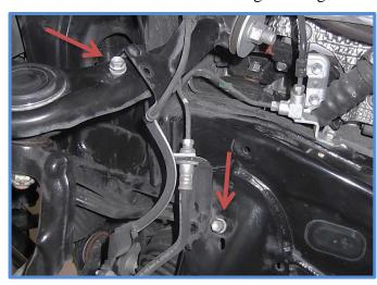
4. Remove the three nuts from the upper mount, lower the jack and remove shock. Remove shocks from both sides before attempting to install new shocks.
