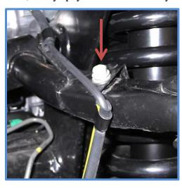
3. Keep a jack under the lower control arm on the side you are working on while disconnecting suspension components. Disconnect upper A-arms (A), tie rods (B), and lower shock mounting bolts (C).
