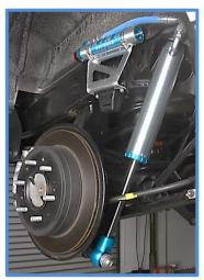
Important Note: The rubber bushings on your King shocks are different from each other. Make sure the taller bushing is on the bottom next to the body of the shock as shown. The silver washer between the rubber bushings represents the material thickness of the upper shock mount. It's important to tighten the nut only until the rubber bushings start to compress. There should be approximately 1/8" of the mounting pin protruding above the nut..
