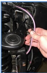
3. Unbolt the ABS/brake line bracket on the spindle using a 12mm wrench or socket
