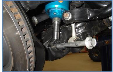
Check the clearance of the spring (with shock at full extension) with the bump stop pad/bracket. You may need grind the bracket slightly so the spring or spring plate does not contact anything at full extension.
