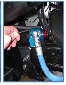
16. The plastic guard can be trimmed to fit around the hose fitting and reinstalled or you can simply remove the guard completely. Photos below show examples of both.
