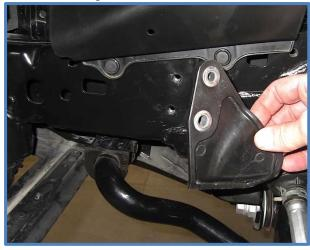
13. Pull the two plastic push pins from the plastic guard and flip up to install reservoir bracket and reservoir.
