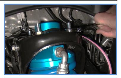
11. Install the lower mounting bolt and tighten to factory specs.
