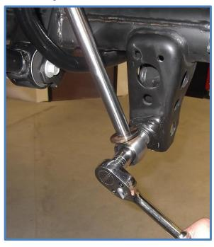
6. Install reservoir brackets. First mount the reservoir clamps to the reservoir brackets using the 1/4 x 1/2" button head cap screws as shown below. Use red locktite and tighten with a 5/32 Allen wrench.
