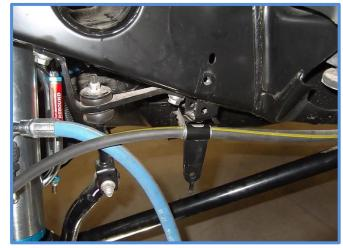
10. Slide reservoir into reservoir bracket. Install the 1/4 x 1" socket head cap screws, leave loose for now you will have to adjust the hose and tighten clamps last.
