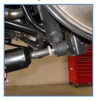
2. Remove upper nut using a 22mm wrench. You may need to hold the top of shock with large pliers.
