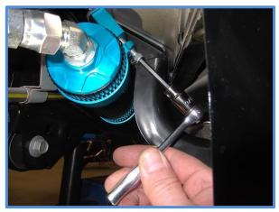
11. Place loop clamp on hose as shown and use the provided 8mm x 25mm flanged head bolt to mount the loop clamp and the parking brake cable holder to the frame.
