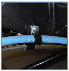
12. Adjust hose: Make sure hose and or fittings are not in contact with frame or body mount. You can rotate the shock and or the reservoir or adjust hose as needed for a clean install. Shocks are built as close as possible to the required hose clocking but some adjustments may be necessary.
