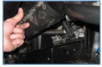
15. Bolt reservoir bracket to frame using the factory bolts and plastic piece as shown below.
