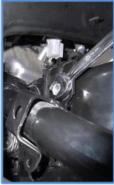
7. Remove the four nuts from the upper mount using a 14mm wrench or socket.
