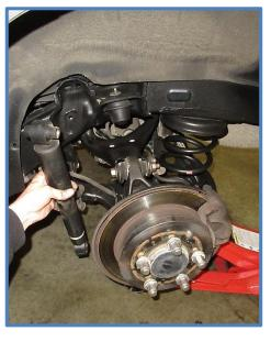
3. Slide the provided spacer onto the lower mounting stud as shown, then place the rod end on the stud. Install the provided bolt with washer and tighten to factory specs. Do not reuse the factory bolt.
