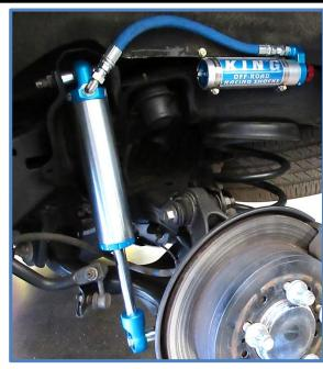
**REAR:** With the vehicle on level ground, block the front tires. Using a floor jack, raise the rear end and support the frame rails with jack stands for safety. **NOTE: Never work under an unsupported vehicle.**
