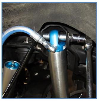
5. Install reservoir brackets – You will need to drill two holes in the pinch seam to mount reservoir. Measure back (7 inches) from the shock mount as shown. Measure up 5/16 and center punch. Drill 1/4" hole.
